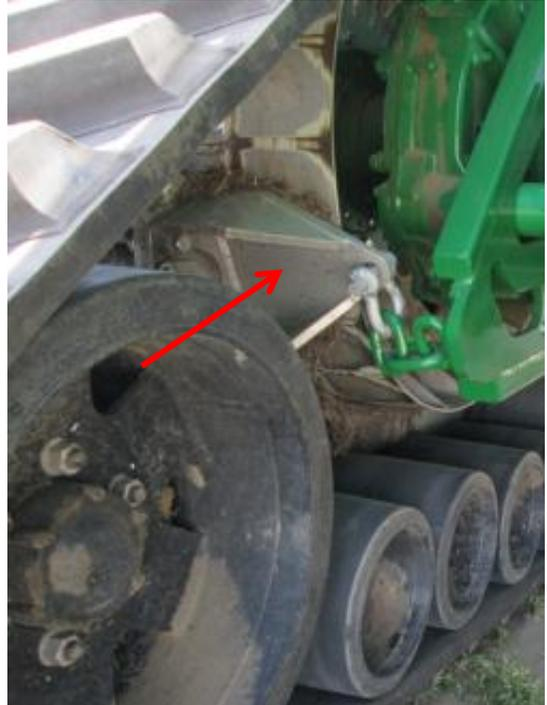
8. Identify if the combine has axle extensions installed or not. Combine axle extensions are a factory option when purchasing a combine. Although, a large portion of the combines in North America have the axle extensions, it is still important to verify that the combine has the axle extensions installed to determine best installation of the CTS.
