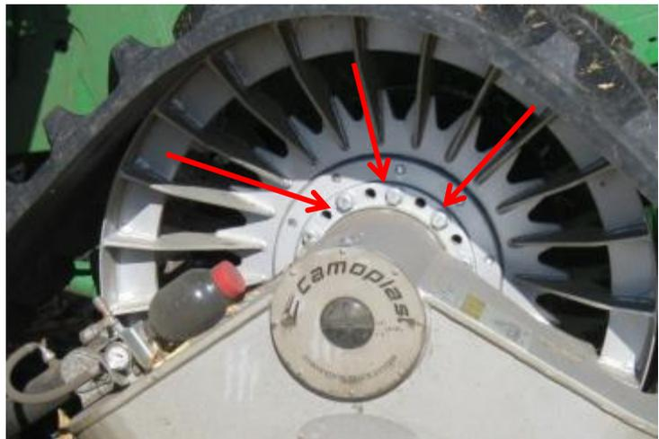
17. After 1 hour of use, retorque mounting bolts to 370 ft-lbs (500 Nm) for combines using M20 bolts and 500 ft-lbs (670 Nm) for combines using M22 bolts. Repeat hourly check until no further bolt rotational movement occurs.
