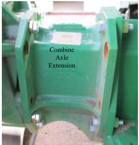
9. Install the track system onto the combine axle. Take care that the front of the track is on the tensioning cylinder side.
